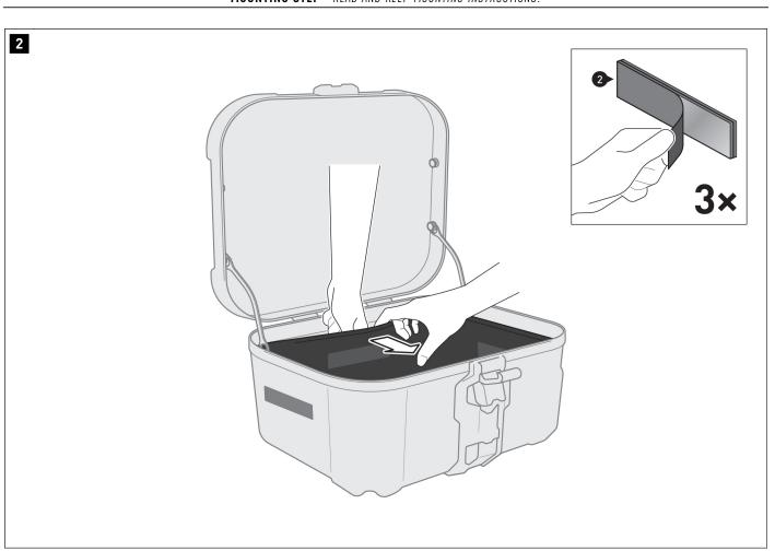
Once the inlay (1) is in place, carefully pull the sides of the inlay (1) away from the wall of the DUSC. Make sure to hold the inlay (1) in place. Peel the backing paper off the Velcro strips (2) ...
